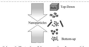
Schematic illustration of the preparation of nanoparticles
