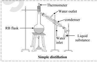
ii. It consists of round bottom flask fitted with a cork having a thermometer.
