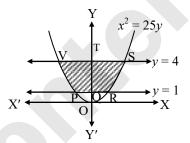
Given equation of the curve is  $x^2 = 25y$  $x = 5\sqrt{y}$ ...[::In first quadrant, x > 0] Required area = area of the region PRSVP = 2 (area of the region QRSTQ)  $= 2 \int x \, dy$  $=2\int_{0}^{4}5\sqrt{y} dy$  $= 10 \int_{-\infty}^{4} y^{\frac{1}{2}} dy$  $=10\left|\frac{\frac{3}{y^2}}{\frac{3}{2}}\right|^4$  $=\frac{20}{3}\left[(4)^{\frac{3}{2}}-(1)^{\frac{3}{2}}\right]$  $=\frac{20}{3}(8-1)$  $=\frac{20}{3}$  (7)  $=\frac{140}{2}$  sq. units
